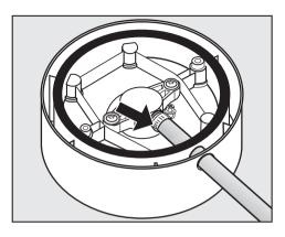
Attach the tube to the outlet underneath the base using the hose clip supplied.
